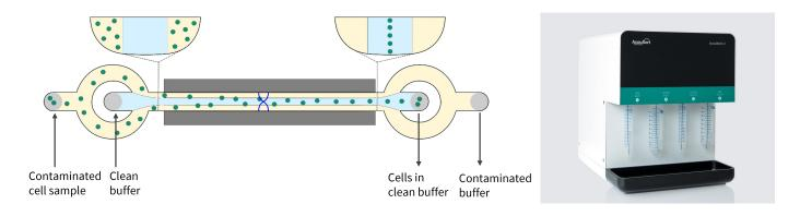
Illustration of the acoustic separation chip that sits inside the AcouWash. In the chip, a piezoelectric transducer generates an acoustic standing wave in the microfluidic channel. The acoustic field moves cells into the clean buffer in the center of the channel, while small particles or contaminants remain in the side fraction.
